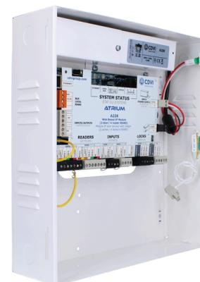
LA CENTRALE C900IP CUORE DEL SISTEMA CENTAUR IN GRADO DI GESTIRE FINO A 2 VARCHI CON 2 LETTORI MULTITECNOLOGIA .
